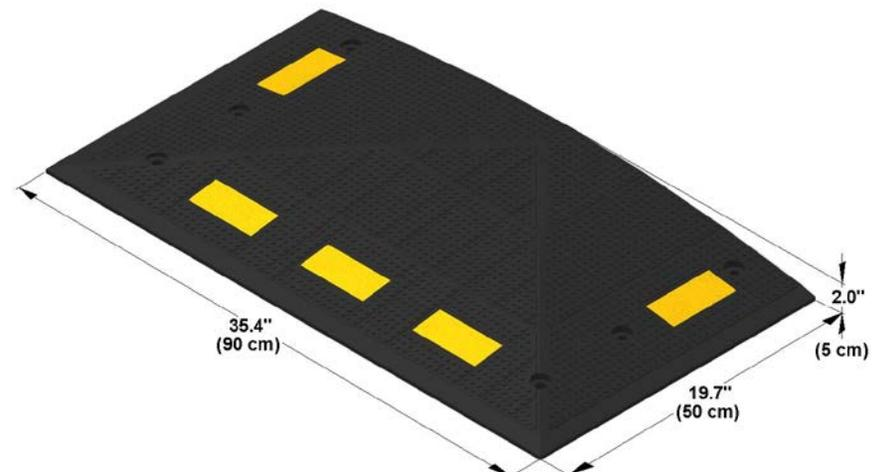
**Installation method:** Each module of the "Safety Rider V" can be installed on asphalt or concrete pavements with six special zinc plated steel bolts 3/8" (10 mm) diameter and 4" (105 mm) long, plastic shields 9/16" (14 mm) diameter 3" (80 mm) long and zinc plated steel washers (supplied with the product) as per following simple installation steps:
